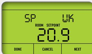
SP (set-point) with room name is visible. The desired room temperature may be set here using the "Up" or "Down" key.
