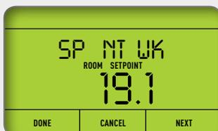
SP NT (nightset-point) with room name is visible. The desired night temperature or temperature when absent may be set here using the "Up" or "Down" key.
