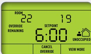
The night temperature is activated and the remaining time that this night temperature is still active is displayed. It is a sort of "kitchen timer", and after the expiry of the set time the automatic program is active again and the screen **A** visible again.
