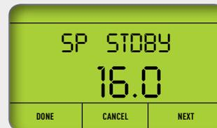
SP STDBY (set point stand-by) is house temperature holiday mode. This is set to 16° C by default. You can change this temperature using the "Up" or "Down" key where 15°C is the minimum.
